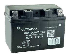
Factory Activated.sealed Ultramax motorcycle batteries ,with acid being completely absorbed into glass mat separators which are sandwiched between the lead plates, giving a sealed and maintenance free battery.
