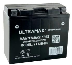
Factory Activated.sealed Ultramax motorcycle batteries ,with acid being completely absorbed into glass mat separators which are sandwiched between the lead plates, giving a sealed and maintenance free battery.
